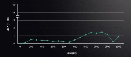
\*After 3,000 hours of QUV testing, the highest dE measured for ECLIPSE profiles is 1.48. A dE from 1 to 2 represents a minimal color difference or a difference that only an experienced observer can detect. ECLIPSE profiles are being continually industry tested for weathering and heat absorption.
